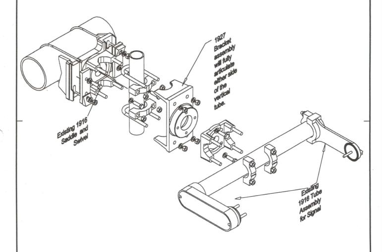
Horizontal signal may be installed at any angle from the mast arm by using the 1927 Assembly.
